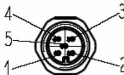
Standard Rexroth 12mm connection cable pin-out
