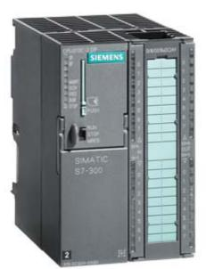
SIMATIC S7-300, CPU 313C-2 DP Compact CPU with MPI, 16 DI/16 DO, 3 high-speed counters (30 kHz), integrated DP interface, Integr. power supply 24 V DC, work memory 128 KB, Front connector (1x 40-pole) and Micro Memory Card required
