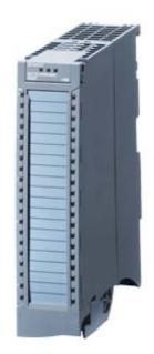
SIMATIC S7-1500, Analog output module AQ 4xU/I ST, 16 bit resolution, Accuracy 0.3%. 4 channels in groups of 4, diagnostics, substitute value incl. power supply element, shield bracket and shield terminal: Front connector (screw terminals or push-in) separately
