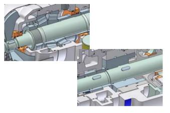
The balance drum device carries the major proportion of the hydraulic thrust. The drum diameters are chosen to minimize the thrust at normal operating point. The residual and additional thrust loads occurring above/below at the normal operating point are carried by the thrust bearing, typically a taper roller bearing.
