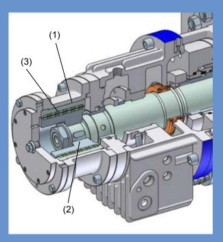
The exclusive Permavor® lift-off device prevents touching and wear of the disk/counter disk during operation at low speed, such as start up and shut down.
