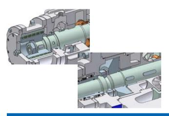
With a balance disk the axial force is completely compensated, no axial thrust bearing is required. Due to the smaller balancing leakage flow, total efficiency of the pump is higher compared to the balance drum design.
